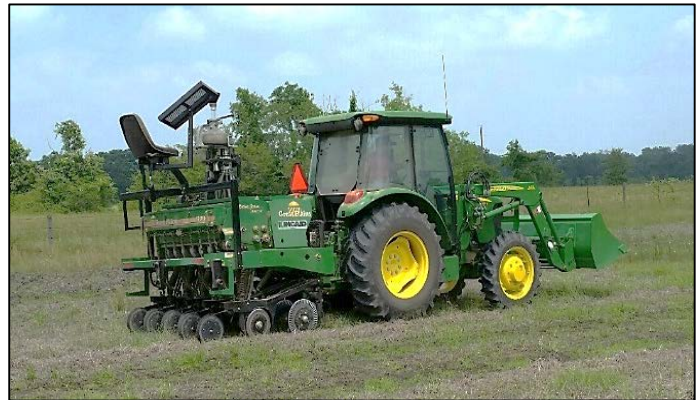
Fig. 3. No till seed drill planting into a seedbed prepared by mowing and herbicide applications.
